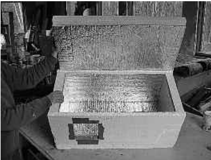
The inside box is made of polystyrene that has good insulating properties.
