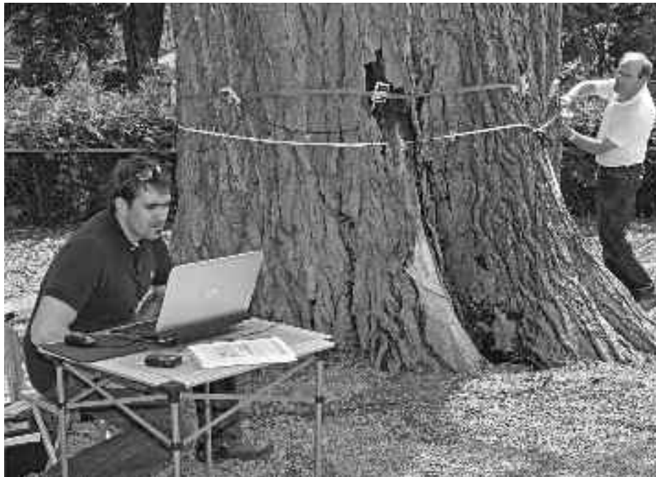
Forestry engineer Luc Nadeau, right, installs sonic sensors to the trunk of the huge, approximately 75-year-old Eastern cottonwood (a type of poplar) located in the Lansdowne dog run. Another engineer, left, monitors the Picus Sonic Tomograph unit, which detects decay and rot inside tree trunks using sound waves. Five to 20 of the sonic sensors were placed around the circumference of the 8-foot diameter tree.
