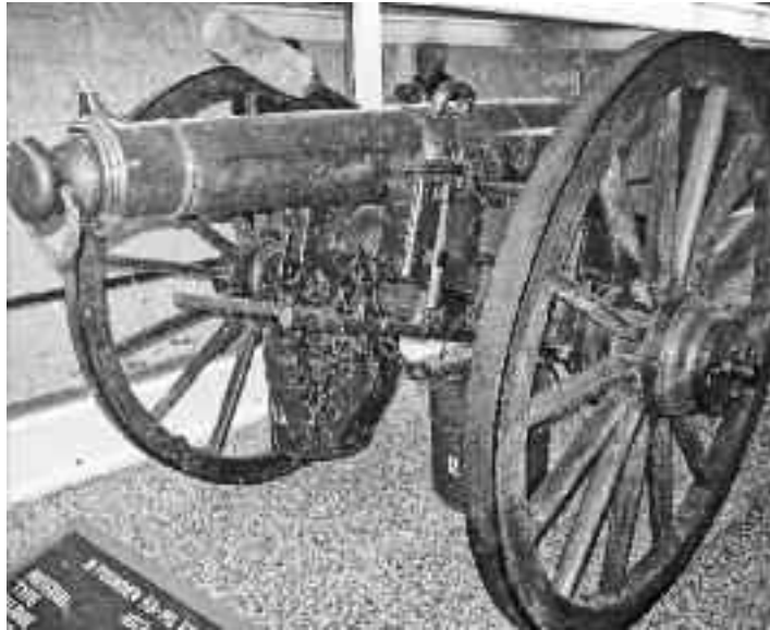
Authentic five-foot diameter wooden wheels on this 9-pounder gun carriage behind glass at Fort Henry, Kingston, are the model for the new wheels in Westmount.
